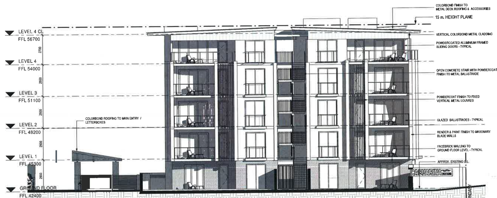
2 EAST ELEVATION - BUILDING A 1:100
